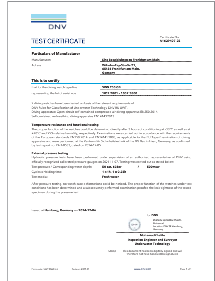
DNV verifies and certifies the pressure resistance of our T50 GB to a diving depth of 500 m and the temperature resistance and functionality in accordance with the European diving equipment standards EN250 and EN14143.
