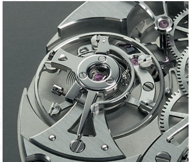
The regulator system of the hand-wound calibre UWD 33.1: In accordance with the functional principle of a swan-neck regulator, this regulator system enables zero-play precision adjustment of the watch. The six eccentric weights on the balance wheel for precisely balancing the balance system are also clearly visible.
