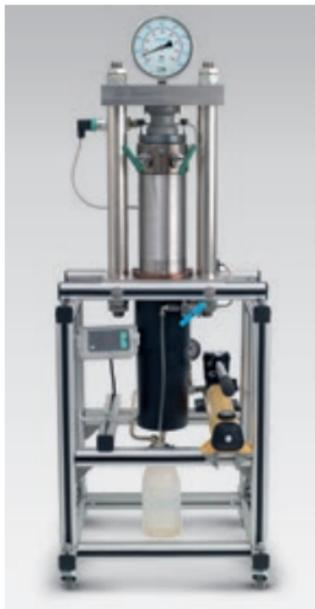
*Image: All of the technical details of our watches are documented by tests. This system of assessment has been specially designed for certification of the pressure resistance of our diving watches by DNV.*
