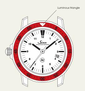
The diver's bezel is a rotatable bezel that can be set to the minute and only be rotated in one direction to prevent accidental adjustment. It has a luminous main marker which can be used in various ways. It can be used to highlight important time periods. Use it, for example, to mark the start of a period of time; the elapsed time can then be read off at a glance at any time.
