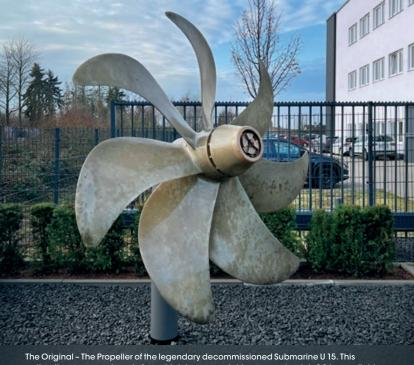
The Original – The Propeller of the legendary decommissioned Submarine U 15. This authentic component made from ship's bronze, weighing approximately 1.1 tons, reliably powered the U 15 above and below water for decades. Today, this impressive propeller proudly adorns our company headquarters.
