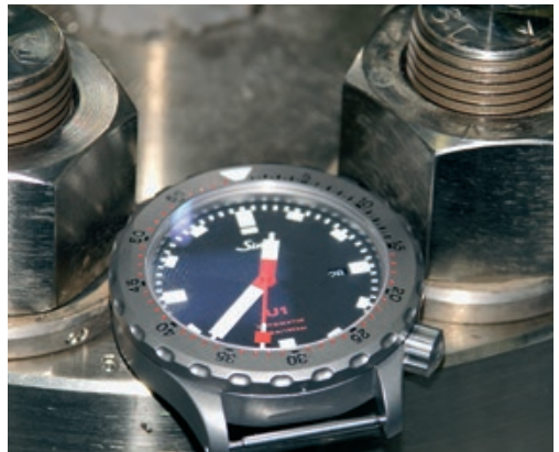
Pressure vessel fitting with 36 mm thread: The U1 easily passed the 100 bar test. 1 bar = 100,000 pascals.
