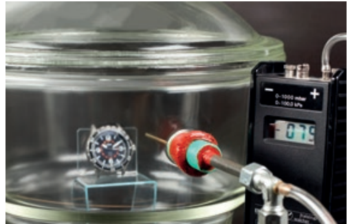
Differential pressure test in a vacuum desiccator: A pilot's watch in accordance with DIN 8330, such as the 857 UTC VFR , must be able to withstand several thousand pressure cycles.
