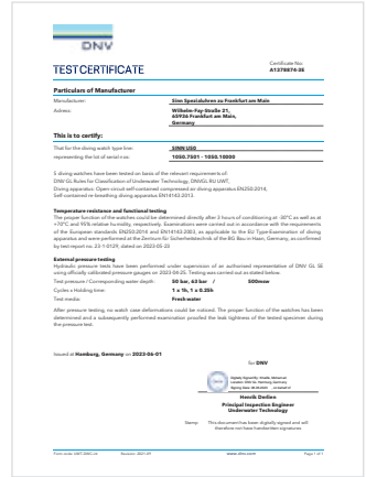
DNV verifies and certifies the pressure resistance of our U50 series to a diving depth of 500 m and the temperature resistance and functionality in accordance with the European diving equipment standards EN250 and EN14143.
