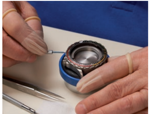
During final assembly, the individual components are pieced together to form complete cases, as shown here by the EZM 7 mission timer for the fire service.
