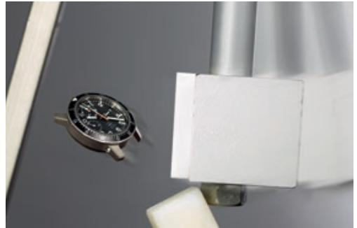
Test system for impact and shock resistance testing. Here, the 103 Ti IFR is being tested.
