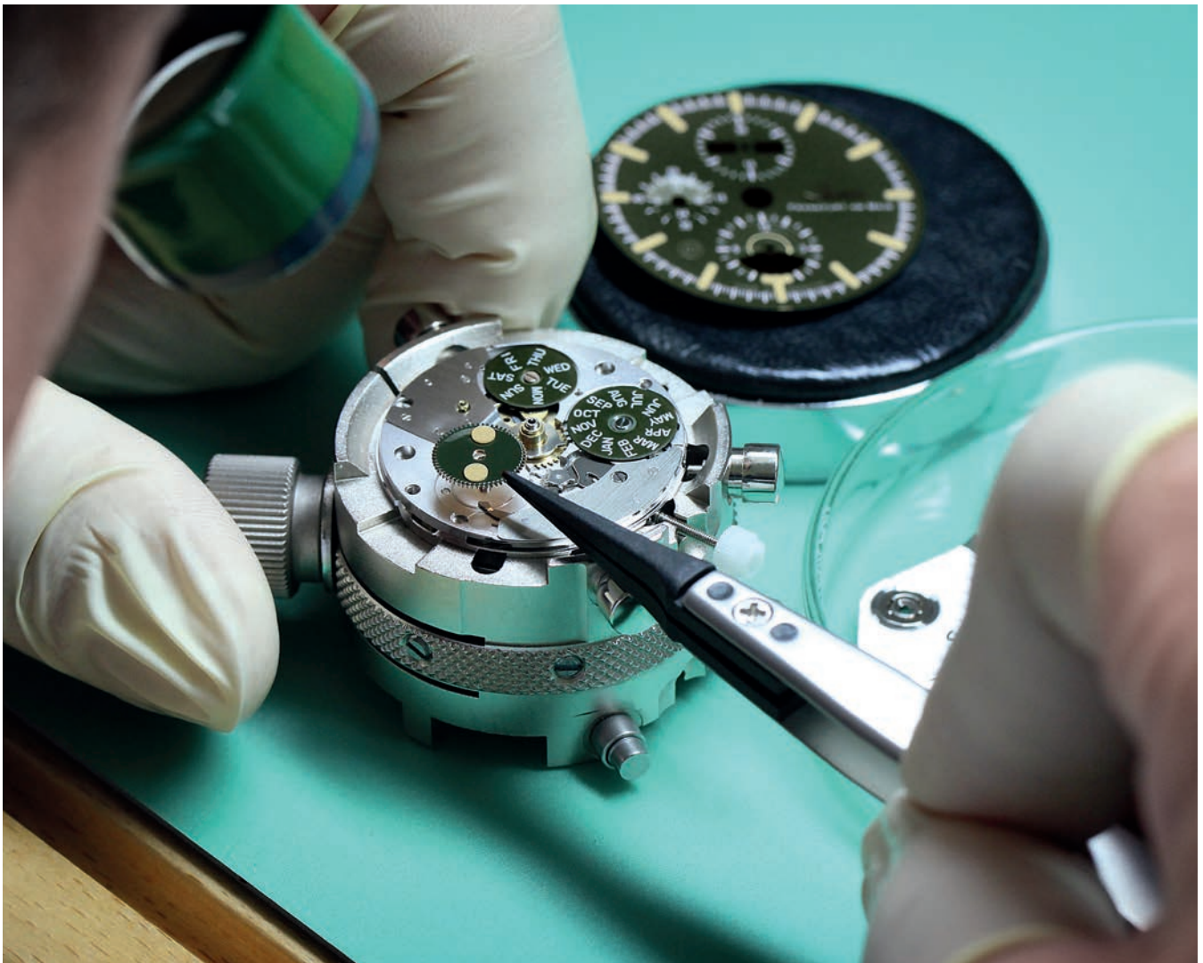
Precision craftsmanship down to the finest detail: attaching the moon disc on the HUNTING WATCH 3006 also requires the ultimate concentration.
