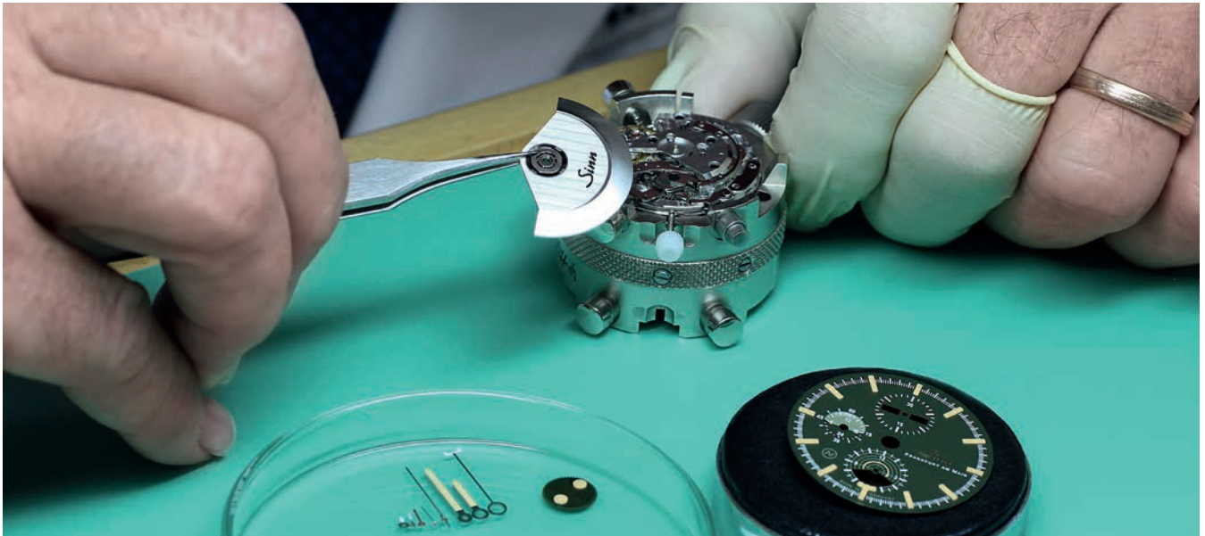
The assembly of the winding rotor completes the exquisitely decorated movement of the HUNTING WATCH 3006. The delicate hands, the dial and the moon disc are ready for assembly.
