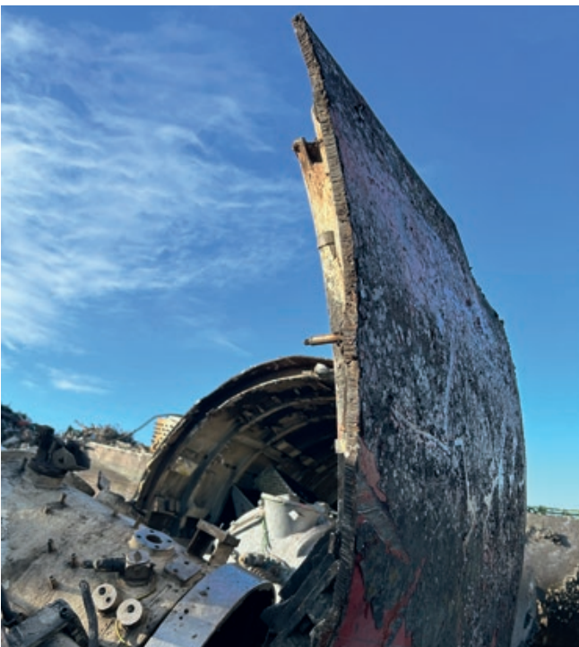
The inner wall thickness of a Type 206 submarine is much thinner than you might think thanks to a sophisticated stiffening structure.
