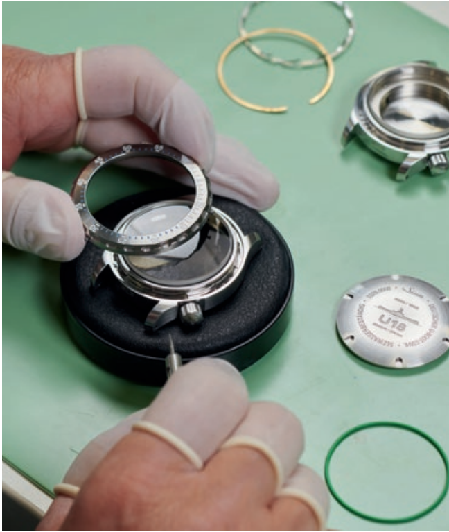
A case receives its components, such as the rotating bezel, middle, back, sapphire crystal, crown, seal, snap and spring rings.
