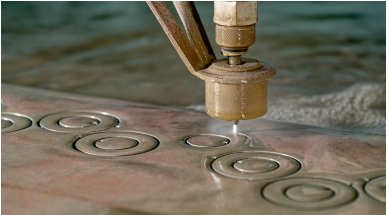
A water jet cutter is used to cut out the blanks for the case back and middle and the rotating bezel from the straightened plates of German Submarine Steel.
