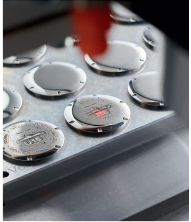
The intricate engraving on the screwed back, made using a precision laser system.
