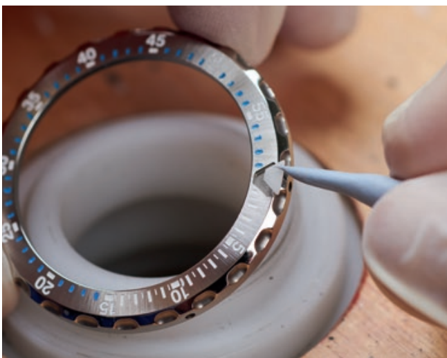
The illuminated triangle of the rotating bezel is set and bonded by hand.
