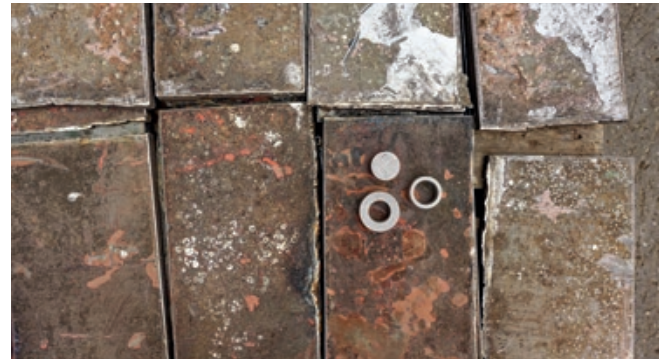
Straightened steel plates from the U 15 submarine and the resulting blanks in various dimensions.
