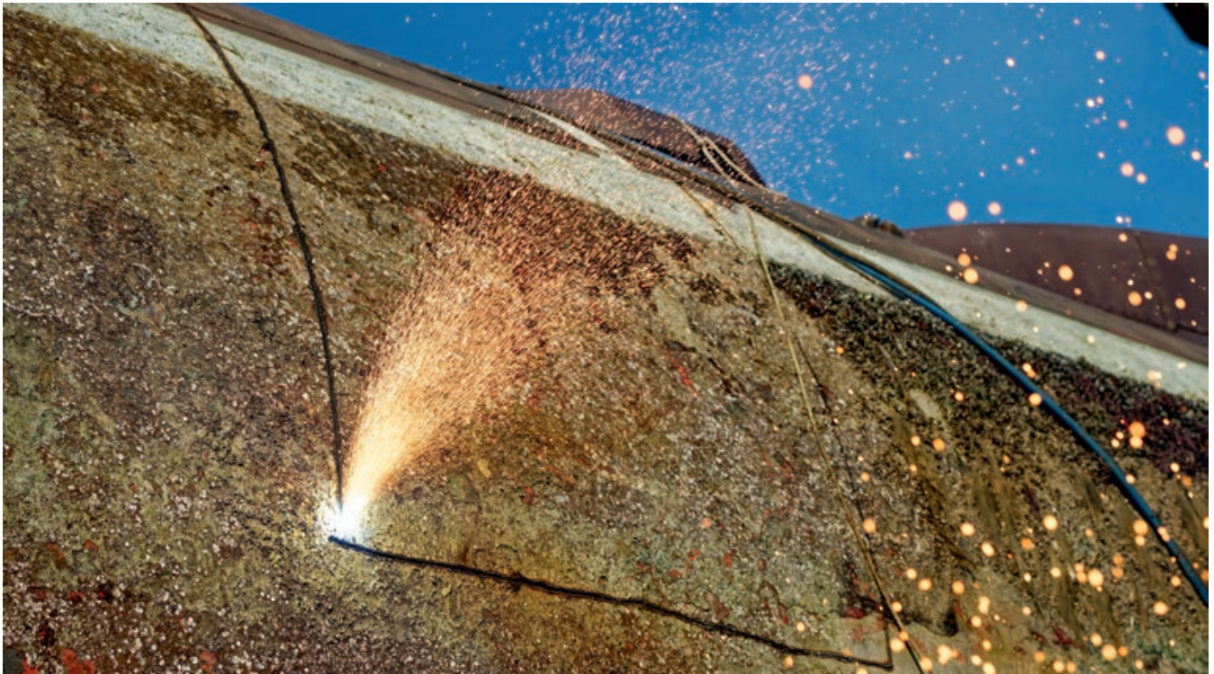
The first step in the recycling process at KSH: A flame cutter is used to cut out steel plates from the U 15's hull.
