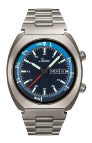
the triangular mark 'HW 1' on the rotating bezel. This can be taken for example from a tide table or tide calendar. The hour hand can then be used to read off the current water level on the rotating tide bezel of the 240 St GZ. You can also read off the expected relative water levels for any given time up until the time of the next high tide, which is then shown at the position 'HW 2'.
